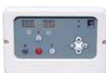
**Control panels for steam generators with electric heater.** The "Operating" light, steam room temperature display, working hour countdown, automatic disinfection function (ozone) can be observed outside the panel.
