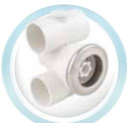
**"SP-1434ASS" Model Massage Jet.** Water and air connection Ø 50, PVC, 2" inlet included. Frame is stainless steel. Recommended flow; 1,5 m<sup>3</sup>/h - 7 mwh
