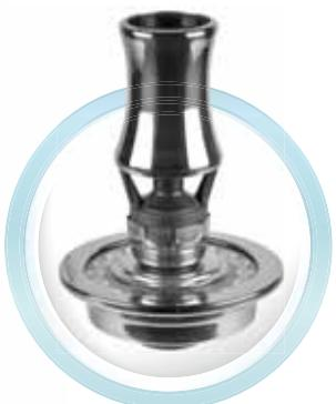
**"SPOT 05"** Underwater light to be coupled with fountain nozzles. 304 quality stainless steel body and single union. 15° light angle with Power LED. Different Adaptors are used for different size nozzles (for exp. 1", 1,5", 2"). For this reason nozzles diameter should be mentioned during the order. (Nozzles are NOT included to the price). 13 different light models are available. With 50 cm Cable.
