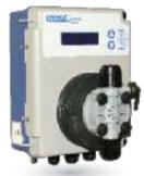
1 solenoid dosing pump Proportional Dosing FWM (Frequency with Modulation) ; Flow rate 5 l/h ; Pressure 5 bar ; Wetted parts Body in PVC, membrane in PTFE
