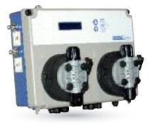
2 solenoid dosing pump Proportional Dosing FWM (Frequency with Modulation) Flow rate 5 l/h ; Pressure 5 bar ; Wetted parts Body in PVC, membrane in PTFE
